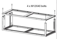
If during assembly of the side upright the holes are not aligned or if there is a space of 4mm between the uprights, it is required to loosen the bolts and reassemble.
