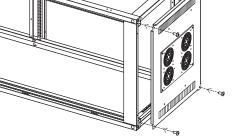
For the cabinet over 800 depth, the fans should be assembled closed to the rear door.
