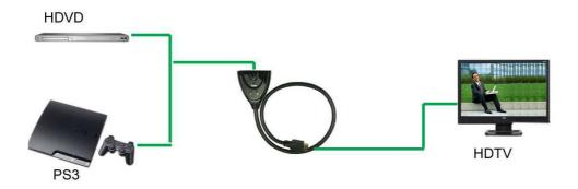
2, You can also connect the HDMI Displays to the two HDMI inputs and connect the HDMI sources to the HDMI male port. Then, press the "select" button to select one HDMI display from two.
