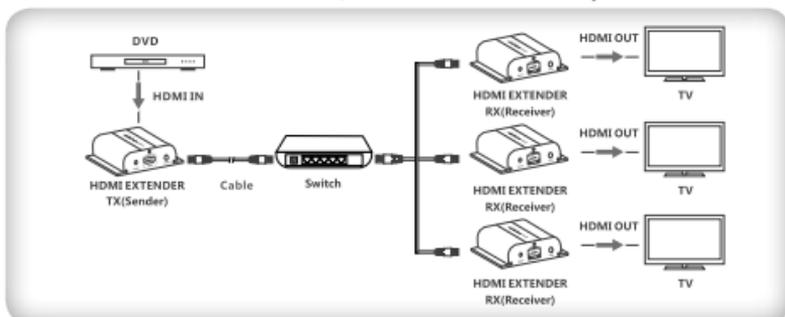
**Note:** Gigabit (1000Mbps) switcher is recommended in LAN transmission.
